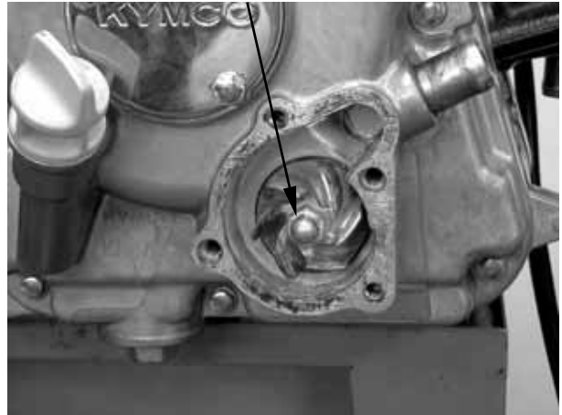
Impeller (Left Hand Threads)
